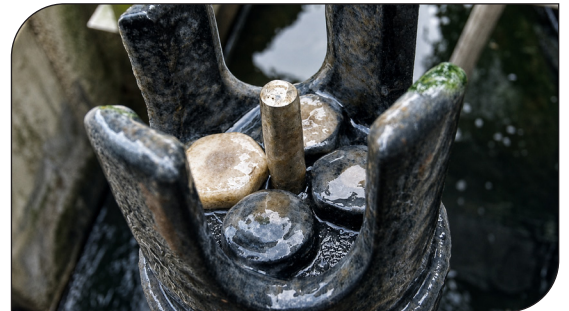
Some buildup was visible after six weeks of continuous operation in the anoxic basin, but the sensor continued to provide usable process measurements.
